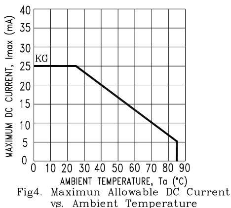
Fig4. Maximum Allowable DC Current
