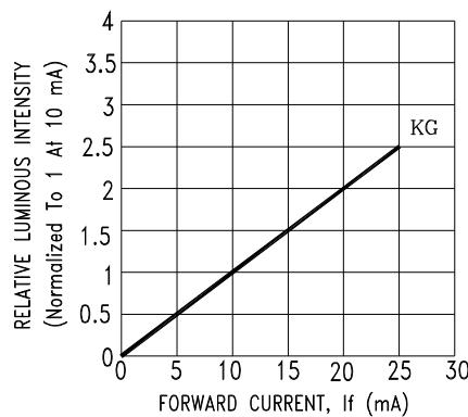
Fig3. Relative Luminous Intensity
