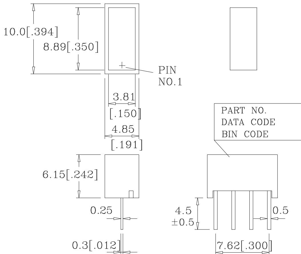
**Note:** All dimensions are in millimeters. Tolerances are  $\pm 0.25$  mm (0.01") unless otherwise noted.
