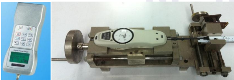
Fig 5-1 Push & Pull Test Equipment 推拉力测试设备
