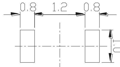
Note: Tolerances unless mentioned  $\pm 0.1$ mm. Unit = mm
