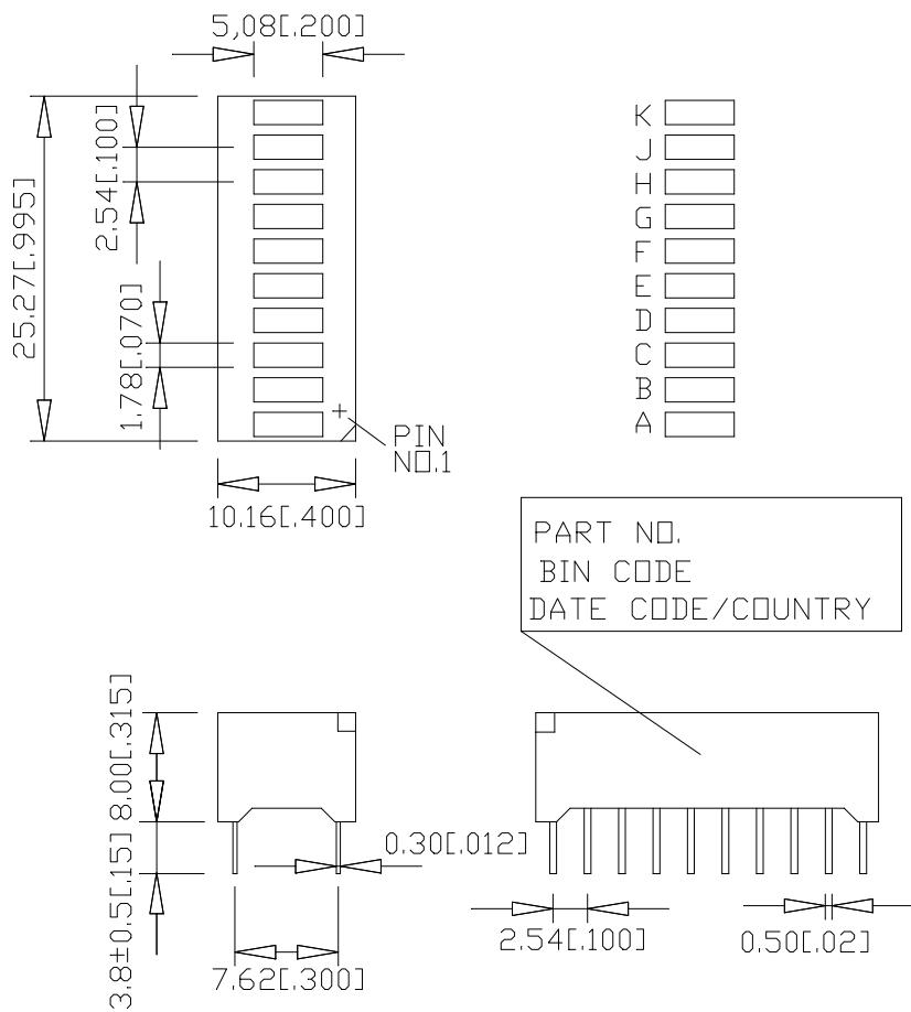
NOTES: 1. All dimensions are in millimeters. Tolerances are  $\pm 0.25$  mm unless otherwise note.
