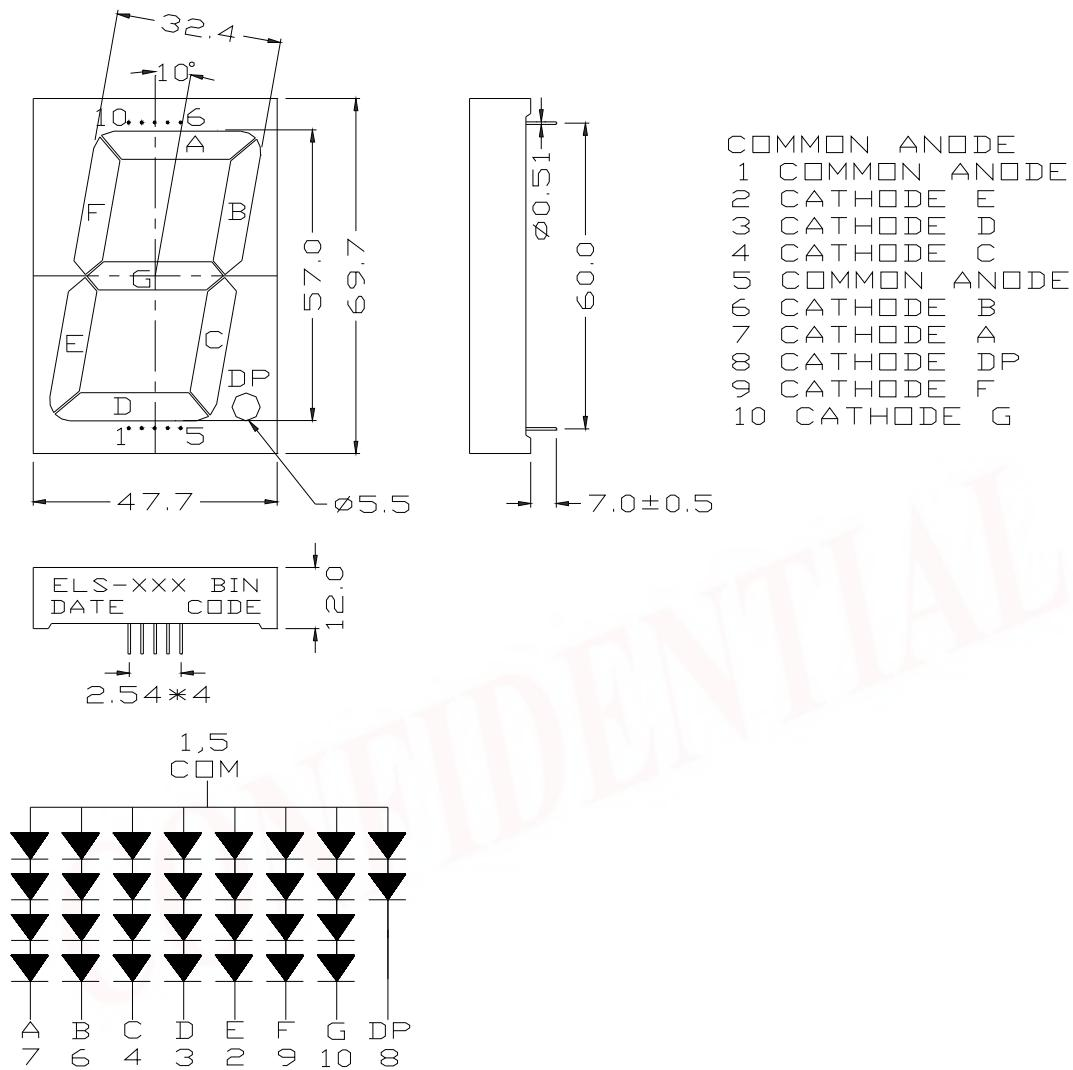
Note: Tolerances unless mentioned  $\pm 0.25$ mm. Unit = mm
