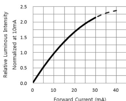
Fig. 4 RELATIVE LUMINOUS INTENSITY
