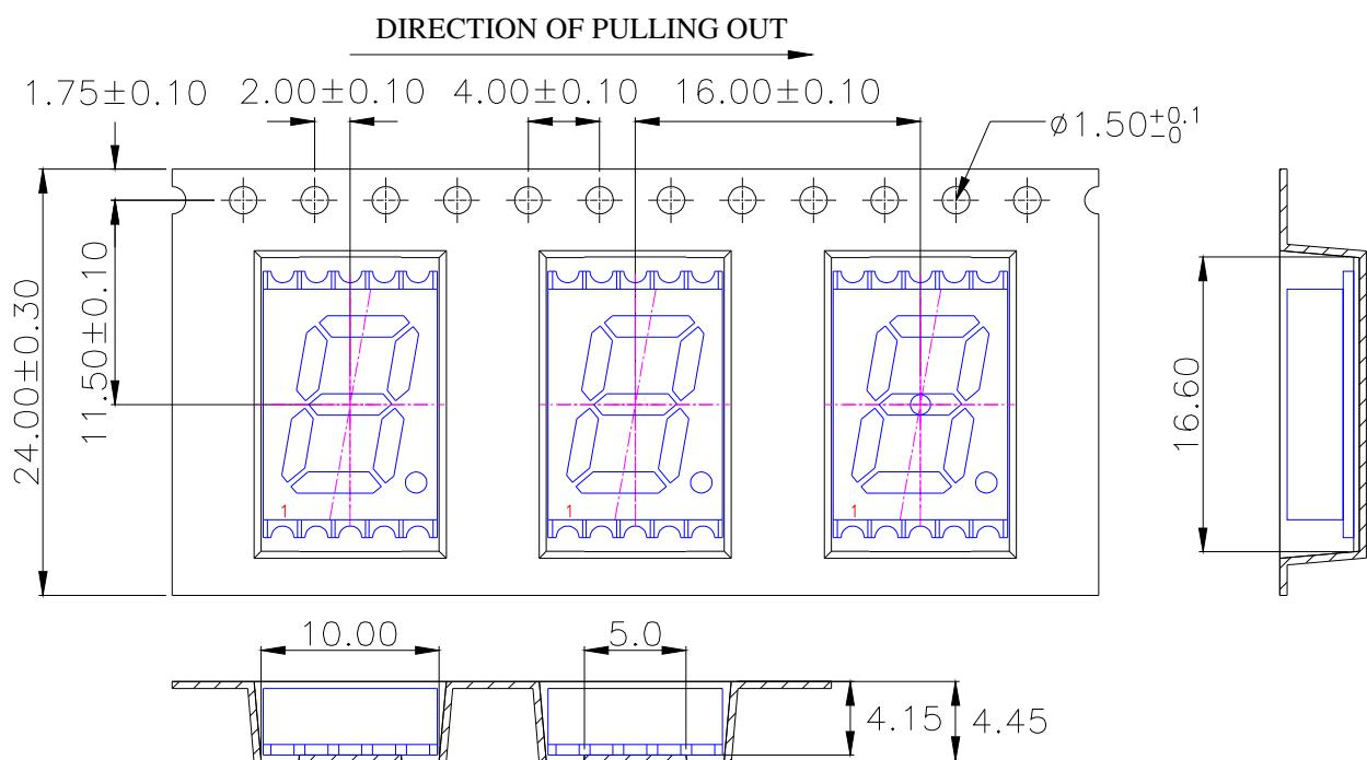
1. 10 sprocket hole pitch cumulative tolerance  $\pm 0.20$ .
