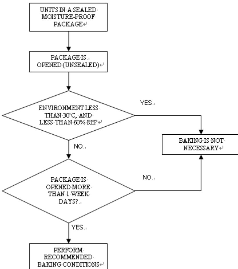
If the parts are not stored in dry conditions, they must be baked before reflow to prevent damage to the parts. Baking should only be done once
