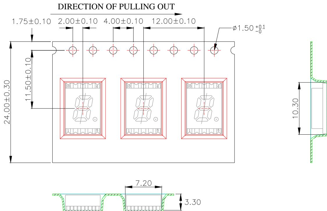
1. 10 sprocket hole pitch cumulative tolerance  $\pm 0.20$ .
