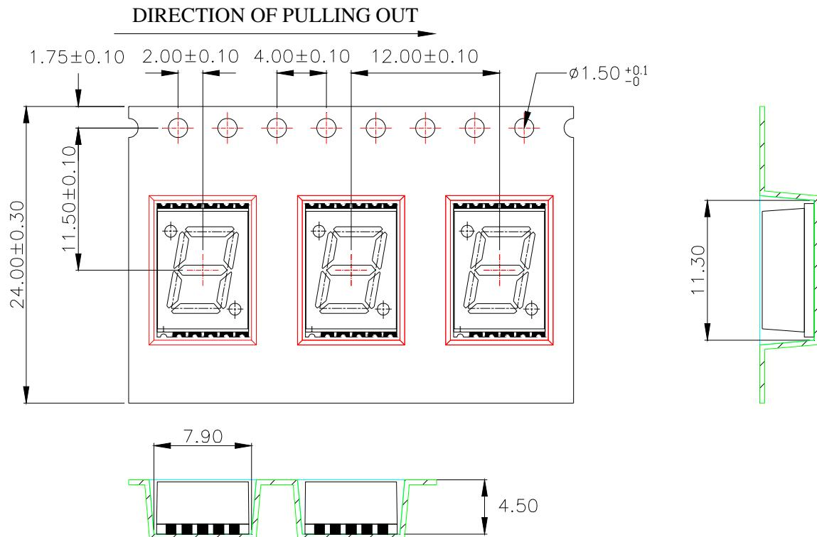
1. 10 sprocket hole pitch cumulative tolerance  $\pm 0.20$ .
