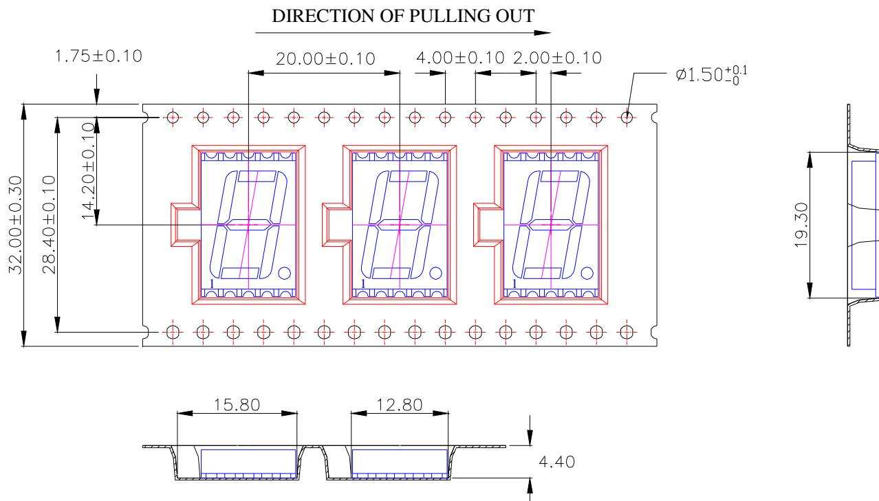
1. 10 sprocket hole pitch cumulative tolerance  $\pm 0.20$ .
