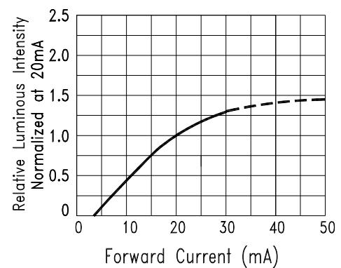
Fig.4 Relative Luminous Intensity
