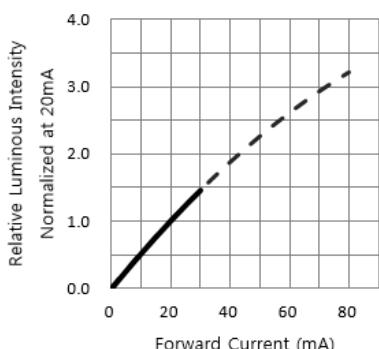
Fig. 4 RELATIVE LUMINOUS INTENSITY
