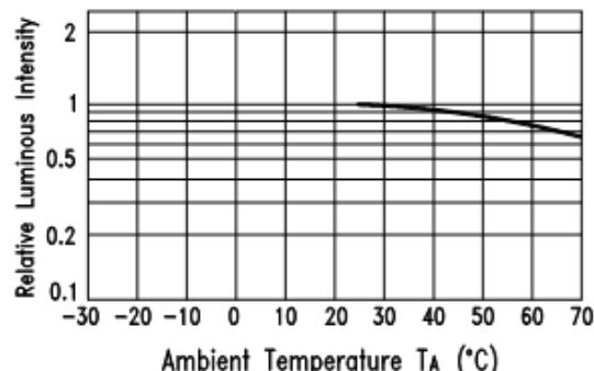
Fig.5 Luminous Intensity vs.
