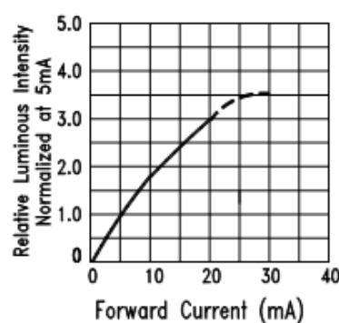
Fig.4 Relative Luminous Intensity
