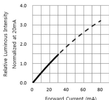
Fig. 4 RELATIVE LUMINOUS INTENSITY
