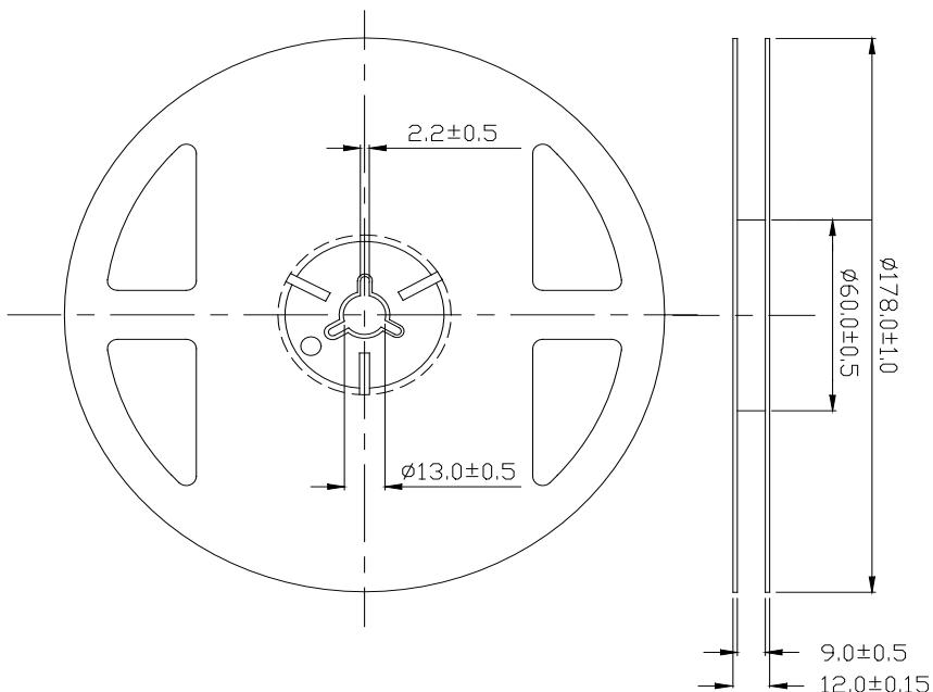
**Note:** The tolerances unless mentioned is  $\pm 0.1\text{mm}$ , Unit = mm
