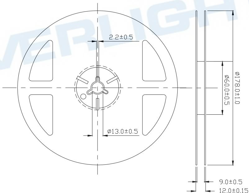
**Note:** Tolerances Unless Dimension  $\pm 0.1$ mm; Unit = mm
