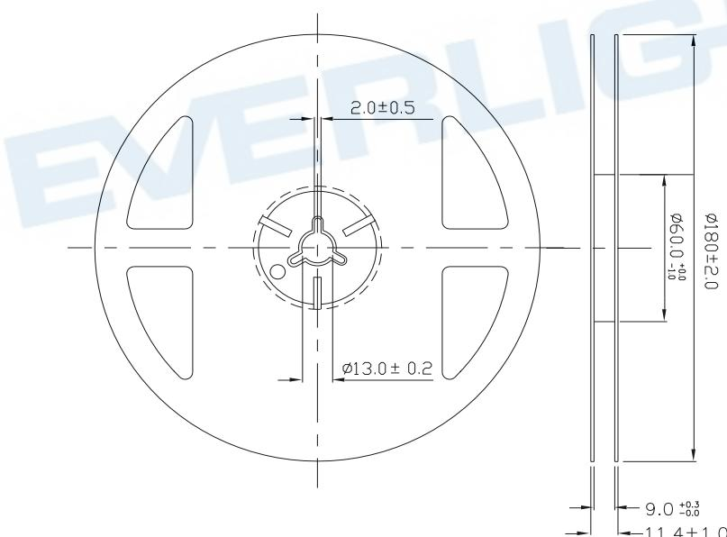
**Note:** Tolerance unless mentioned is  $\pm 0.1$ mm; Unit = mm
