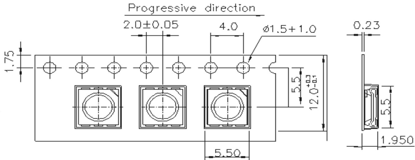
Note: Tolerances unless mentioned  $\pm 0.1$ mm. Unit = mm
