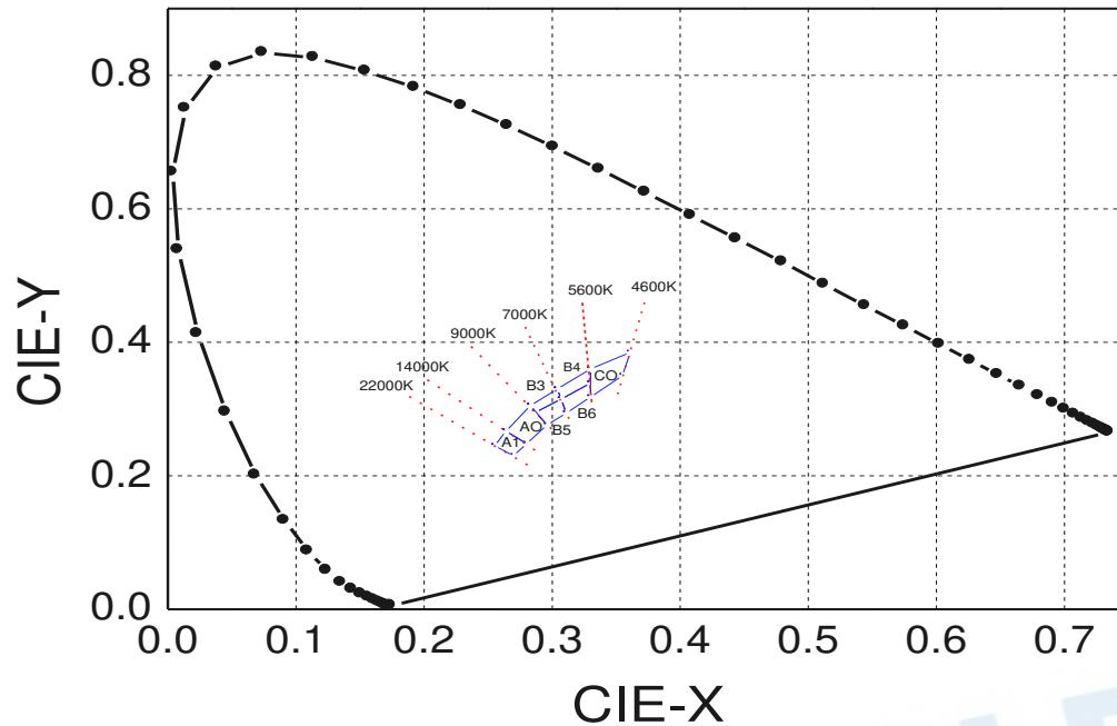
Color Ranks ( $I_F=20\text{mA}$  ,  $T_a=25^\circ\text{C}$ )
