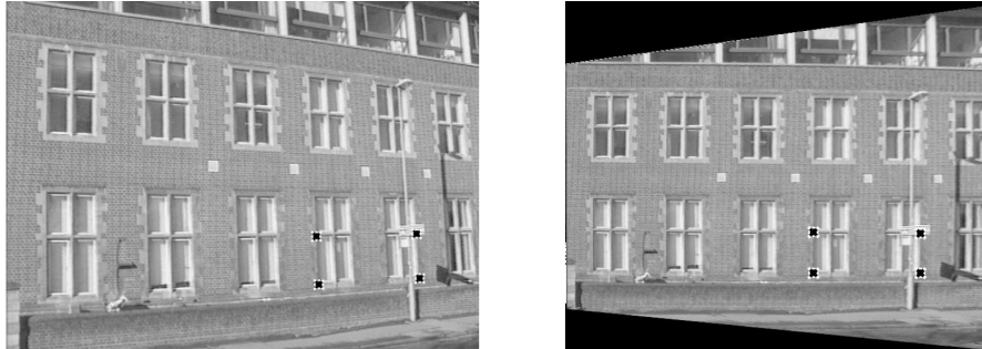
Figure 6: Illustration on how a projection transformation can remove tilting and rotation [9].
