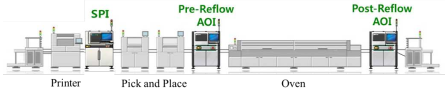
Fig. 2. Surface mount technology line in the laboratory.
